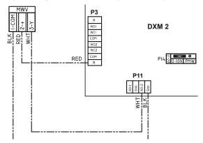
For MWV option, place jumper on 0-10V pins. Ensure actuator direction switch is set as shown.
